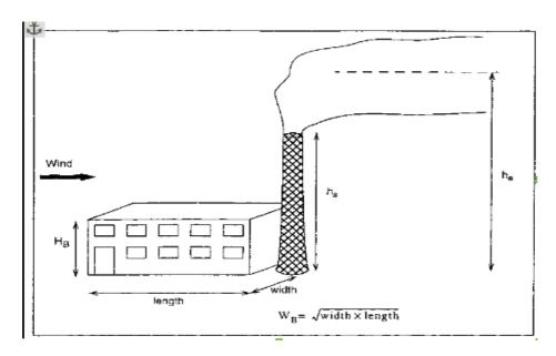
Figure 2C.2 Parameters of interest in the downwash calculation. Find  $\xi$ = min (H<sub>B</sub>, W<sub>B</sub>).
