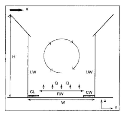
Figure 2E.1 Principles of air circulation within a street canyon (the upwind side is denoted UW, the leewind side LW, see also notations for house height (H), street width between houses (W) and road width (RW)).
