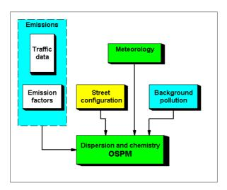
Figure 2J.5. Model structure
