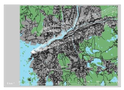
Figure 2.2.2.7 Three stacks with a 2.5 m/s SW wind.
